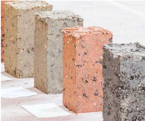
The Three+One system and earth blocks will function as the main components for these structures
