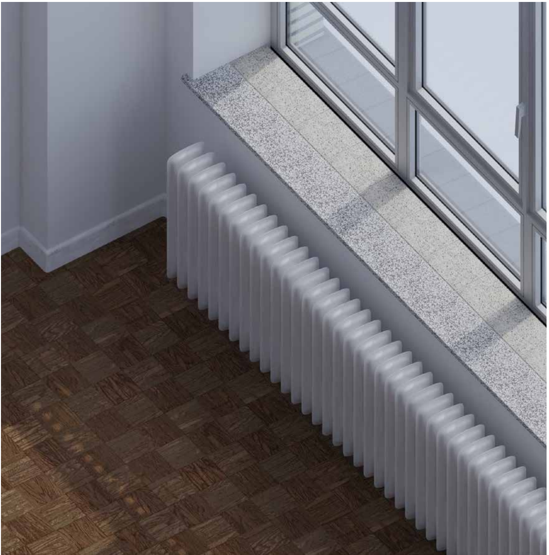
↑ Subtle additions to the existing architecture: 12 cm of cork is added to the facade walls, a new strip for the windowsill and a lime/plaster/sand render protects the insulation and ensures perfect air tightness
